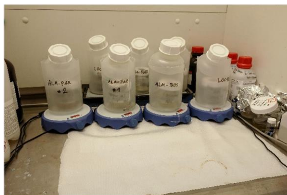
Figure 16: The photo shows the second part of the chemical digestion. Samples are kept in a partly open container under a fume hood due to the exothermic reactions. The samples are placed on magnetic stirrers.
