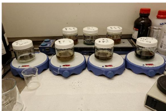
Figure 15: The photo shows seven samples are set to reach room temperature under continuous stirring. This photo was taken right after the first digestion step.
