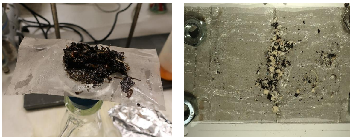
Figure 29: Sample 20170806-ALM-PAR before (left) and after digestion (right). The sample was treated with six rounds of digestion, losing 70 % of the total matter by weight.
