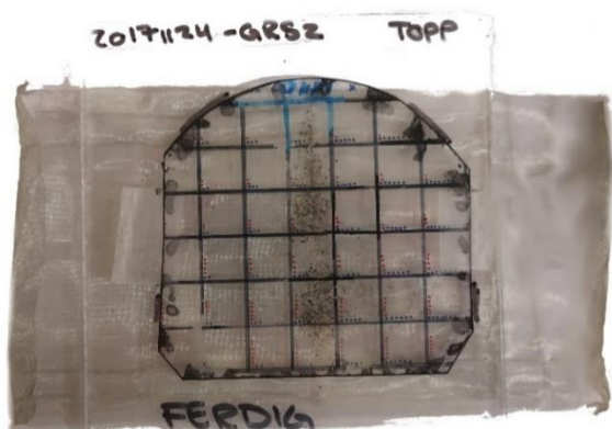
Figure 17: Photo of sample 20171124 – GRS2 locked in place with two acrylic plates. The transparent grid system were attached to the top of the sample.
