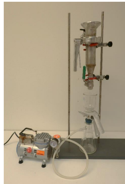
Figure 13: Photo of filtration setup. Extracted sample was filtered onto steel-mesh filters by using a vacuum filtration system. Filter is placed between the filtering cup and the filtering head.
