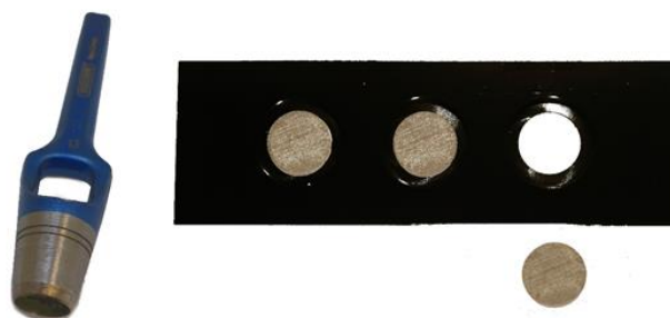
Figure 19: To the right, a hole puncher used for making steel mesh filter fitting the black platform slide (to the right). The diameter of the punched steel mesh filters is 13 mm. The holes in the slide are 10 mm.
