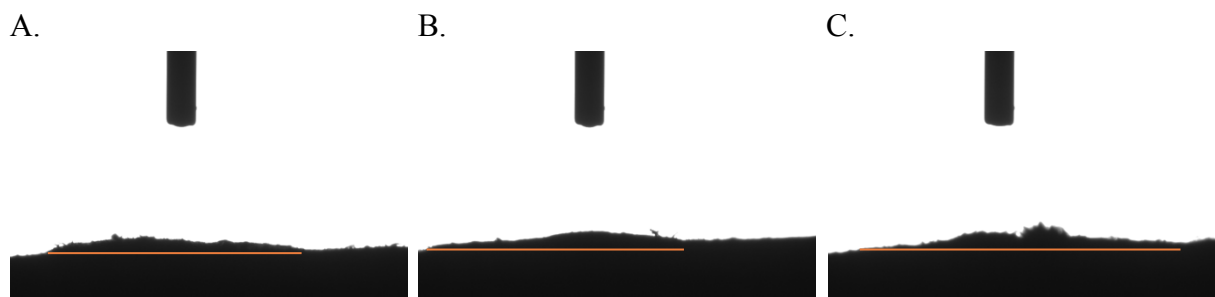
Figure 9.8: The material swelling due to the water drop placed on the surface of the panel with Biotack in the material mix. The swelling is marked by an orange line in each picture. A) The swelling from trial one. B) The swelling from trial two. C) The swelling from trial three.
