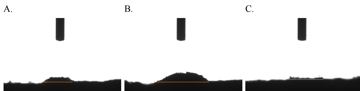
Figure 9.9: The material swelling due to the water drop placed on the surface of the panel with Dextrin in the material mix. The swelling is marked by an orange line in each picture. A) The swelling from trial one. B) The swelling from trial two. C) The swelling from trial three.
