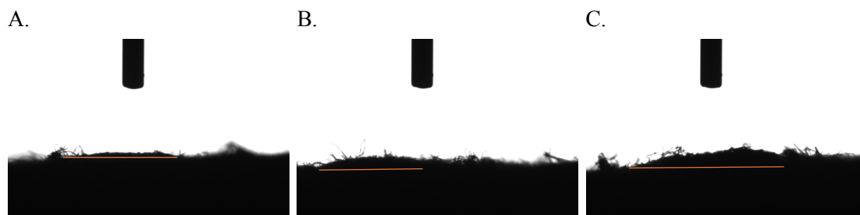
Figure 9.10: The material swelling due to the water drop placed on the surface of the panel with Silicate in the material mix. The swelling is marked by an orange line in each picture. A) The swelling from trial one. B) The swelling from trial two. C) The swelling from trial three.
