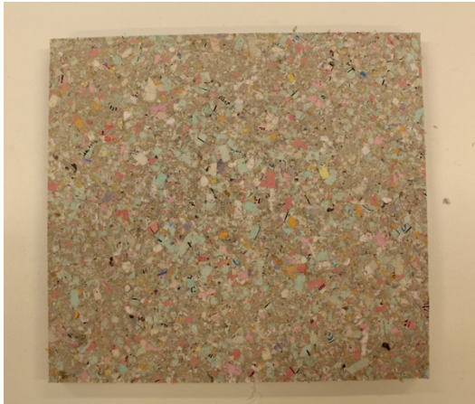
Figure 3.6: The finished product after cooling. A) The panel seen from above. B) The panel seen from the side. (Photo: Authors own)
