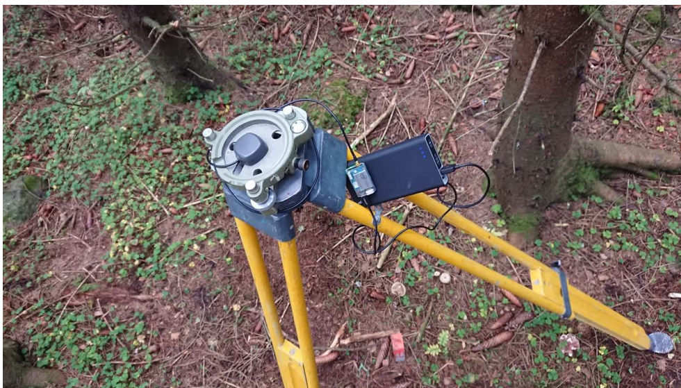
Figure 7: Setup for GNSS data collection, Emlid Reach
