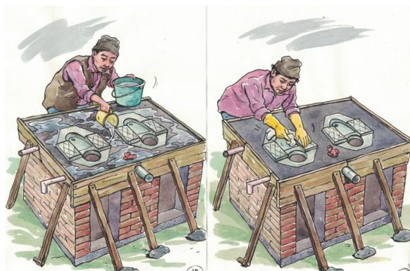
Figure 155: Cleaning of a UDDT (ENPHO, n.d.-a)
