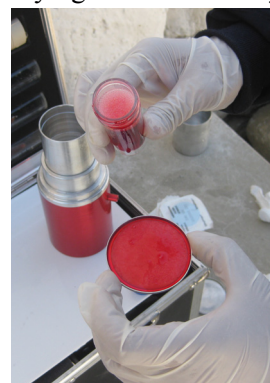
Figure 60: Saturating absorbent pad on petri dish with lauryl sulfate solution for incubation of E.coli
