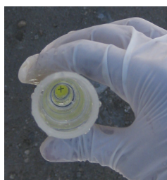
Figure 58: Turbidity test tube with visible cross at the bottom
