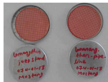
Figure 74: Petri dishes after incubation – no indication of E.coli CFUs which would appear as yellow spots
