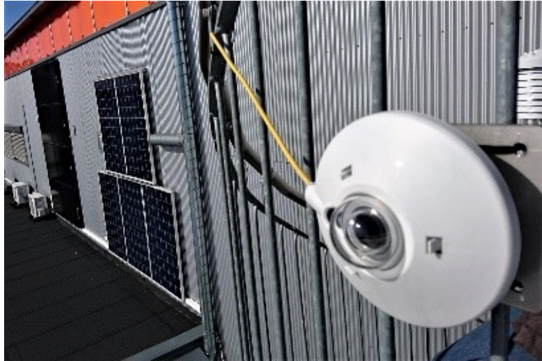
Figure 3.5: Photo of the pyranometer mounted at the test site.
