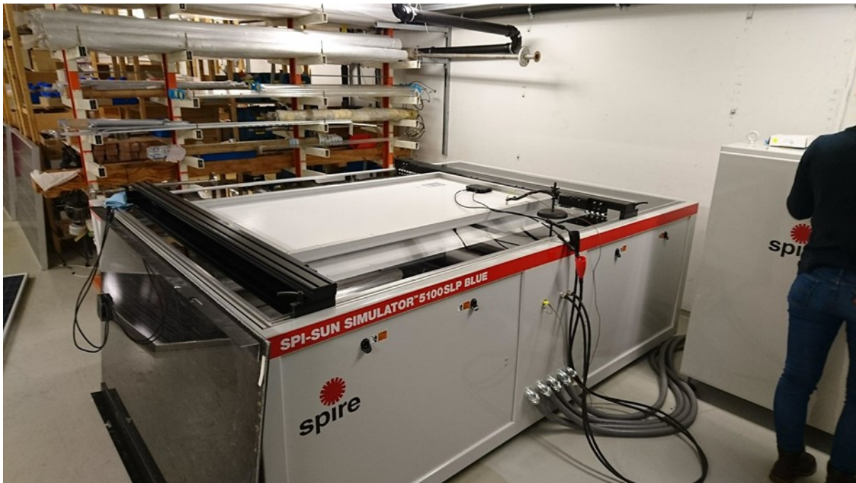
Figure 3.14: The SPI-SUN simulator, 5100SLP BLUE from Spire.
