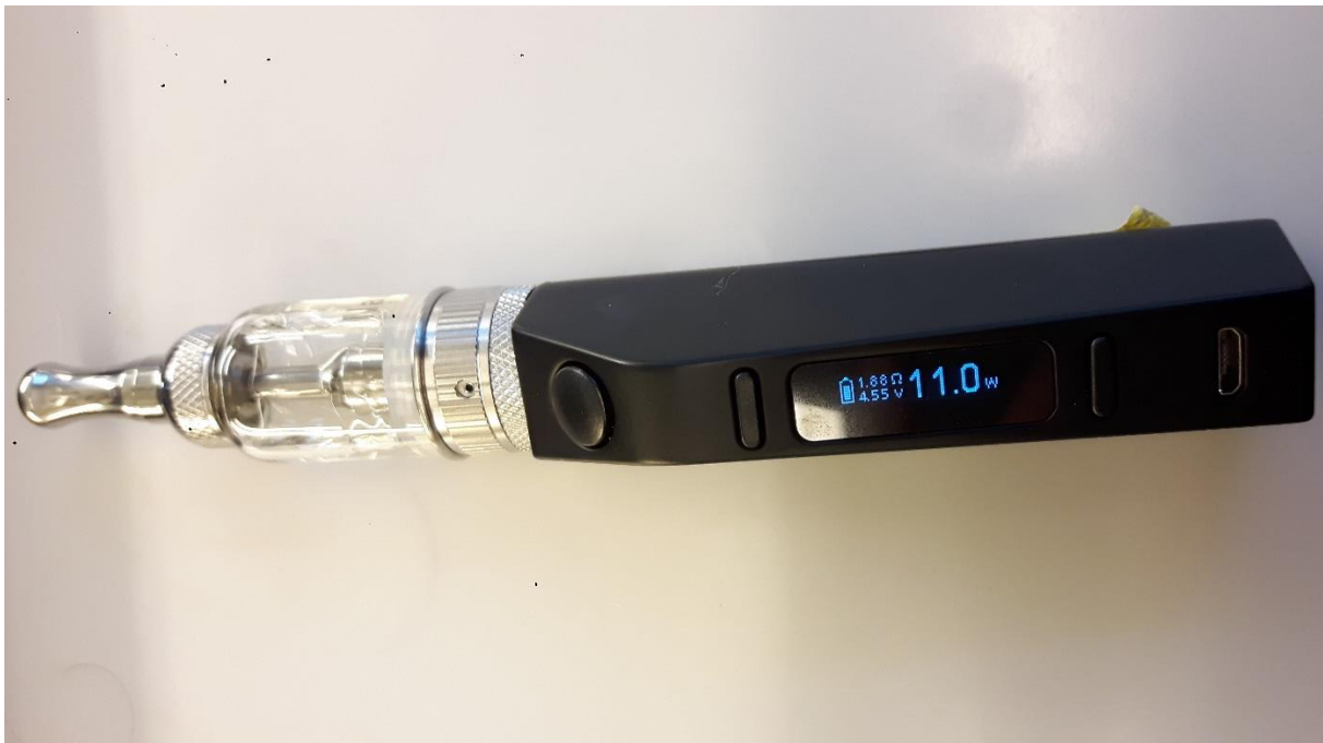
Figure 4. ASTER Eleaf battery with Nautilus Aspire tank system at 11 W, 1 in air flow and an empty tank.
