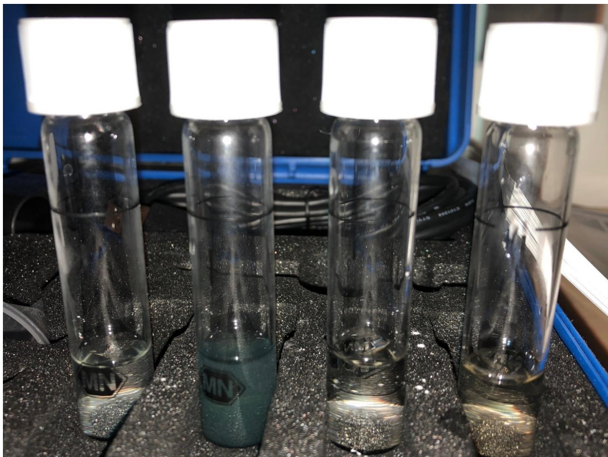
Figure 11: The samples are assigned with numbers from 1 to 4 from left to right. Blue color of sample 2 is obvious probably due to the presence of phenols in the sample (reactants part).
