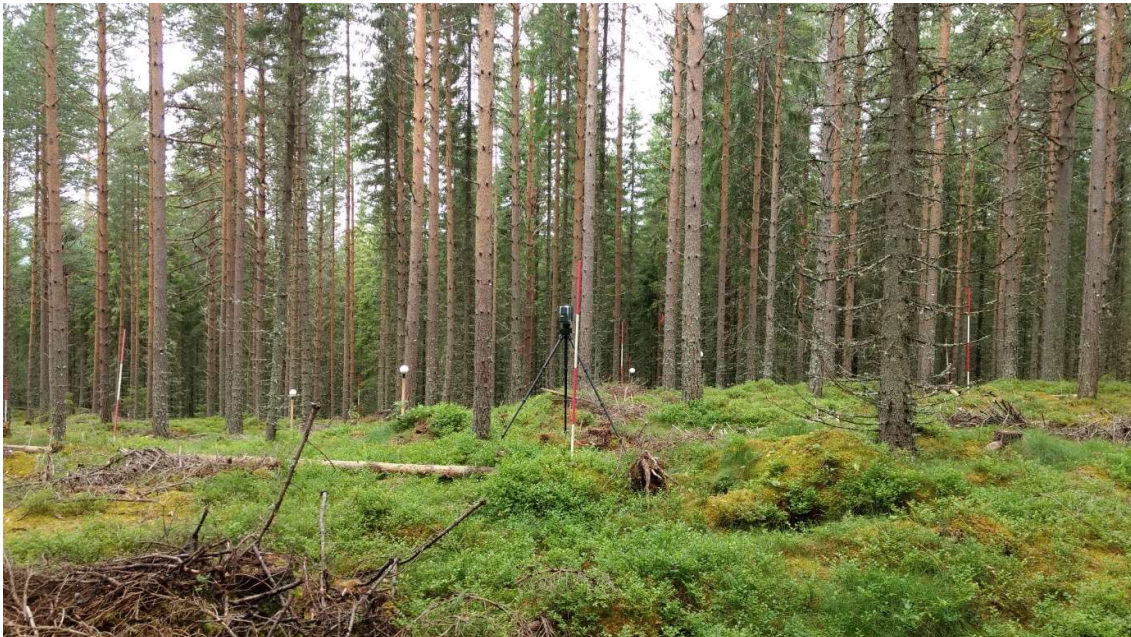
Figure 1. Set up of laser scanner (tripod), scanner positions (red-white poles), and target spheres in one of the sample plots.
