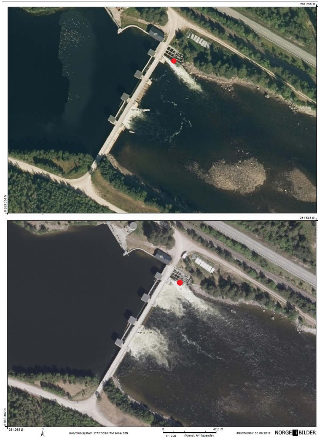
Figure 3 – Aerial photos of dam Høyegga with the fishway located on the east side of the river. The red dot shows the fishway entrance. The two pictures give an impression of how it looks like during low and high flow. Upper: The observed mean observed discharge this day was 33 m 3 /s divided on to spillways. 15 m 3 /s in the tap-spillway and 18 m 3 /s in “flood-spillway 2”. The picture was taken 29.09.2015 (Norgebilder.no 2015). Lower: The observed mean discharge this day was 325 m 3 /s divided on three spillways. 10m 3 /s in the tap-spillway, 141 m 3 /s in the “flood-spillway 1” and 175 m 3 /s in “flood-spillway 2”. The picture was taken 23.07.2013 (Norgebilder.no 2013).
