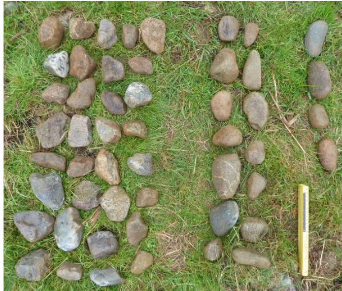
Figure 2.1. Example is of rounding analysis of clasts from a fan lobe deposit in valley 2. Meter-stick for scale 20 cm.
