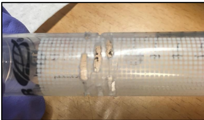
Figure 4: Closeup picture of the holes drilled in the inner tube of the FT-prototypes with membrane.
