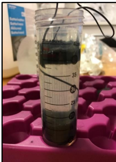
Figure 10: Picture showing the SST-prototype filled with wastewater.
