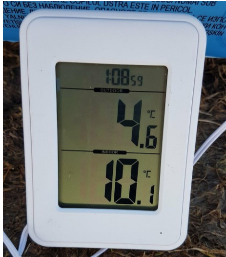
Figure 3.10: Instrument for measuring the water temperature in the pool. Picture taken 10.04.18 at 14.39. Note how the timestamp on the thermometer is incorrect.
