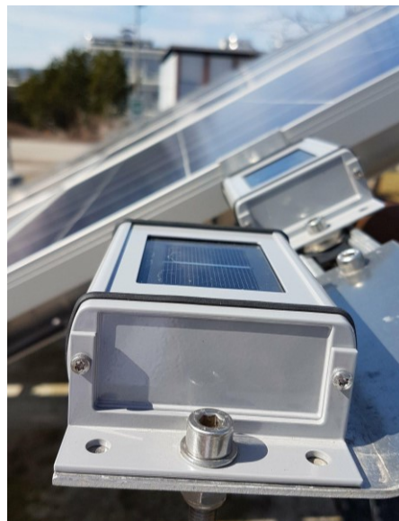
Figure 3.5: The reference cell measuring global horizontal irradiance.
