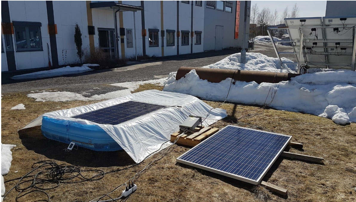
Figure 3.1: The setup of the modules on the test site. The measuring equipment is connected to the grid. The reference cell and temperature sensor are at the PV rack to the right in the figure.
