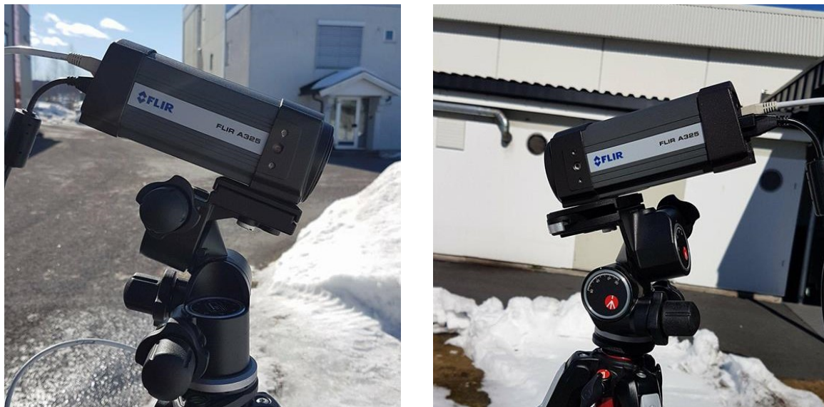
Figure 3.9: IR camera used for mapping the surface temperatures of both modules
