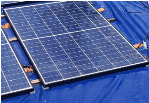
Figure 3.11 (Ocean Sun, by permission): Top: Experimental setup of 12 modules in Singapore. Bottom left: Reference modules lifted by wooden lists. Bottom right: Laminates in thermal contact with the canvas.
