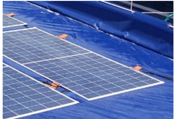
Figure 3.11 (Ocean Sun, by permission): Top: Experimental setup of 12 modules in Singapore. Bottom left: Reference modules lifted by wooden lists. Bottom right: Laminates in thermal contact with the canvas.
