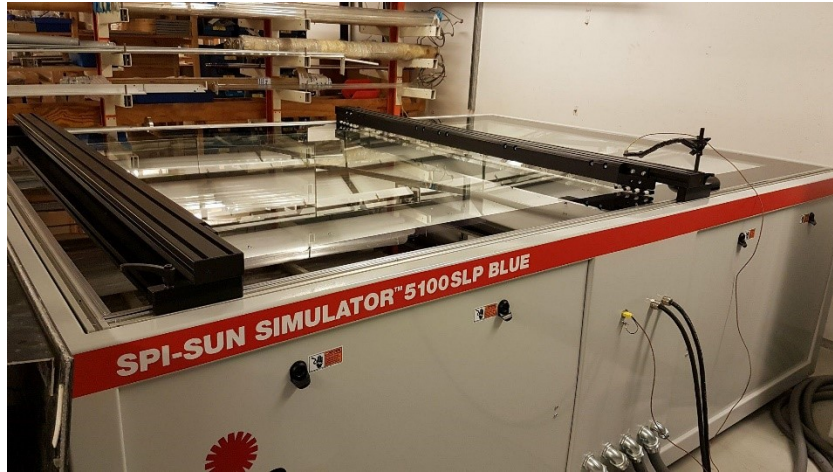
Figure 3.7: Sun simulator from Spire used for flash testing both modules.
