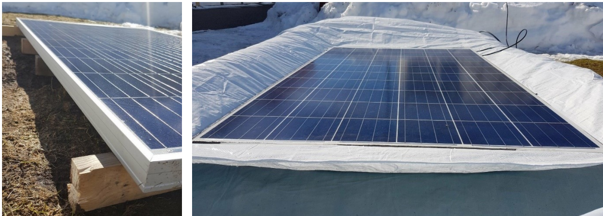
Figure 3.2: Left: Reference module lifted from the ground by wooden lists. Right: Floating module placed on the canvas. The frame is removed from the module.
