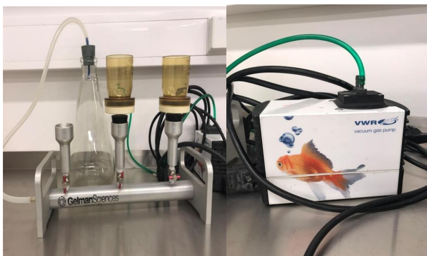
Figure 22: Filter with vacuum gas pump
