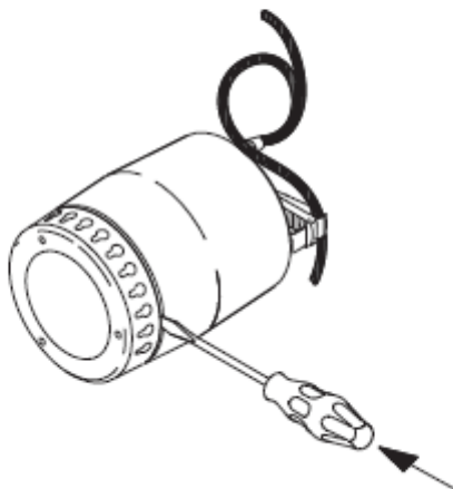
Fig. 10 How to remove the inlet strainer
