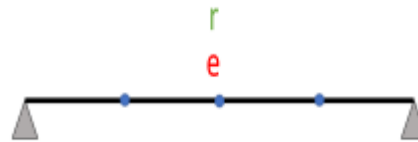
Figure 7.5: Response point and excitation point coincide mid span as the most severe situation.
