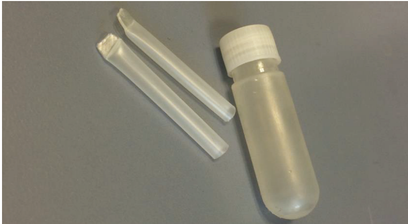
Fig. 11: Shrinking tubes used in HP experiments done in the monovessel unit. Four shrinking tubes (left) were placed in a Cryotube (right) before HP treatment.
