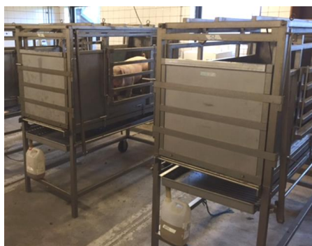
Figure 7. Metabolic crates used for total collection of urine and feces in Experiment 2.
