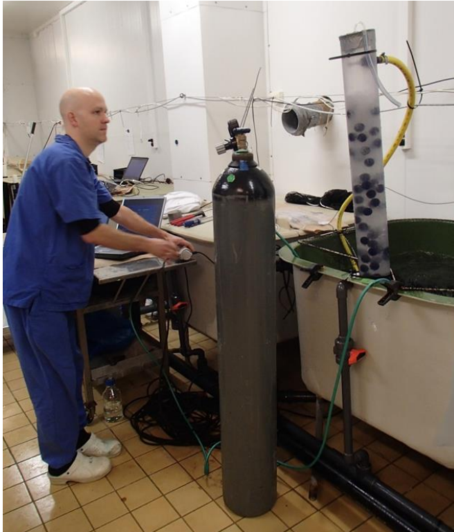
Figure 10. The hypoxia challenge test (HCT). Dr. Sven Martin Jørgensen (NOFIMA, currently FHF) tests the recirculation system and mixture of nitrogen gas into the tank water. Photo: Morten Lund
