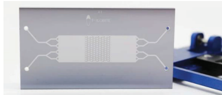
Figure 7. The Trilobite chip model in silicon and glass.
