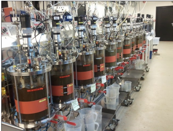
Figure 4.8: The Dolly CSTR of 6 L working volume capacity.
