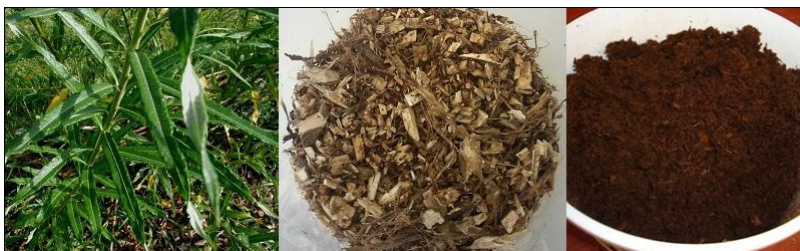
Figure 4.6: Salix viminalis and the chopped sample before and after steam explosion.
