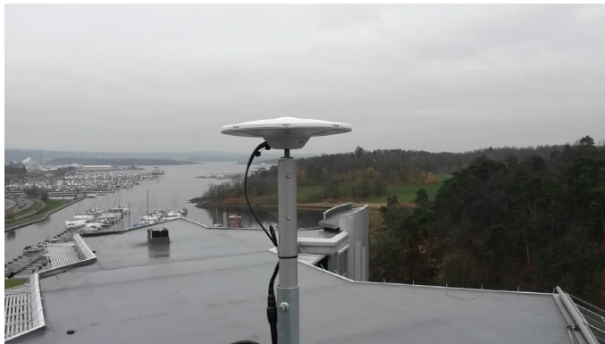
Fig. 8.6: Oslo reference station antenna used for UHD estimation and short- and medium-baseline RTK
