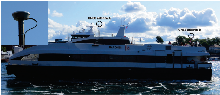
Fig. 8.1: Picture of the Baronen vessel navigating in the Oslo fjord, including a detail on one of the antennas on board.
