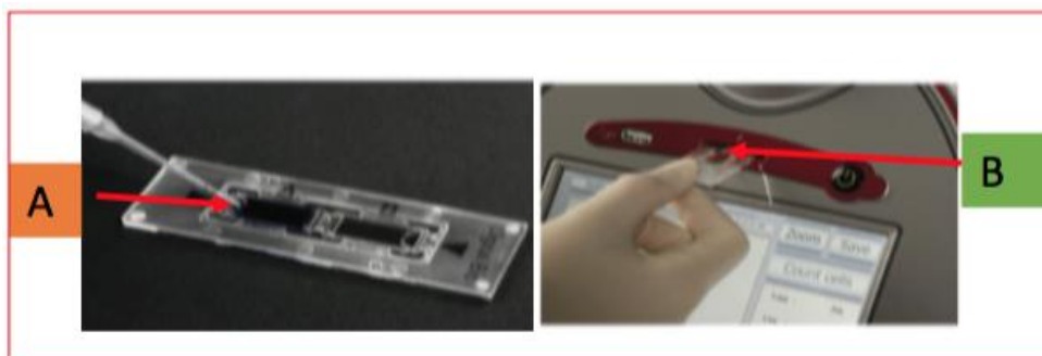
Figure 18: The hemocytometer (left) and the Countess (right)
