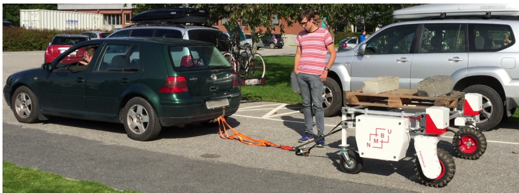
Figure 9. The setup for the traction test. Here, the robot is carrying a 137-kg payload.
