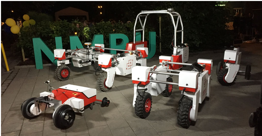
Figure 1. A few examples of robots assembled from Thorvald II modules.
