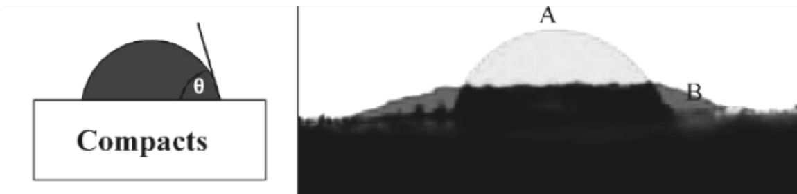
Figure 18: Example of the contact angle measurement by the sessile drop of compact (based on hard wheat flour) method. The initial contact angle (A) and after 3 min (B) (Roman-Gutierrez et al., 2003).
