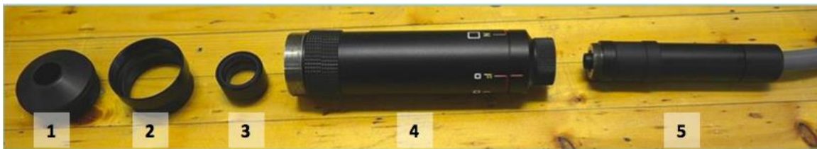
Figure 10: Assembling the video microscope. Items are indicated by numbers: (1) CVM Video probe head, (2) Zoom lens, (3) 20x – 120x basic lens, (4) Contact head adaptor, (5) 60x-420x contact head) (Catargiu, 2015).
