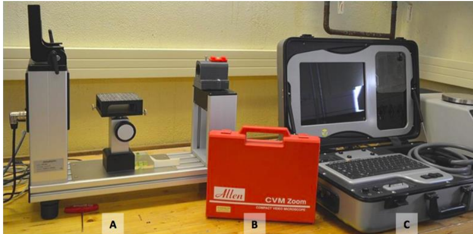
Figure 7: Equipment used for evaluation of under water pellet stability (UPS). Items indicated by letters (A) Krüss Tensiometer, (B) Allen Compact Video Microscope Lenses, (C) Micro Viper Portable Computer) (Catargiu, 2015)
