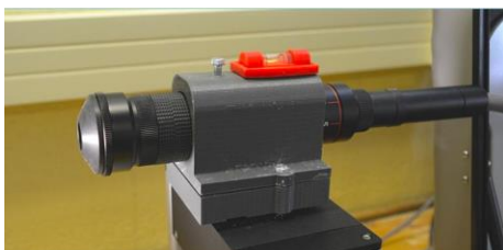
Figure 11: Final view of the assembled and fixed video microscope on the Tensiometer
