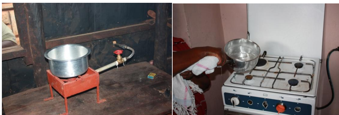
Photo 10: Biogas burners. Left: A locally made metal frame burner. Right: Ordinary gas cooker modified to use biogas. Photo:(Wamwea, 2010).
