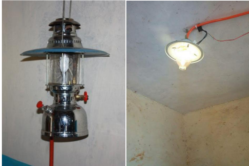
Photo 11: Biogas lamps. Left: The ordinary pressure lanterns. Right: An overhead lamp. Photo: (Wamwea, 2010).
