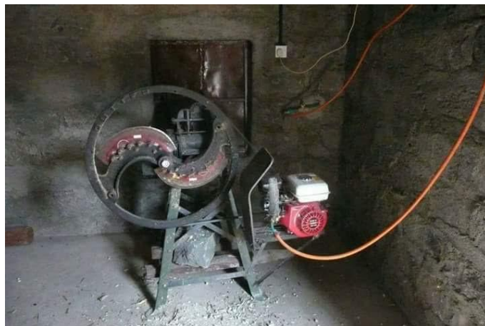
Photo 13: A biogas chaff cutter. Photo: Stephen Ngugi Wamwea
