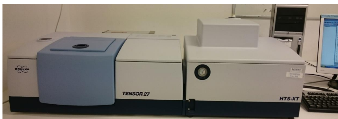
Figure 17. The FTIR instrument with a HTS-XT coupled to it. Photo: Felicia Stehr.
