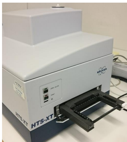
Figure 18. The port where the sample plate was inserted. Photo: Felicia Stehr.
