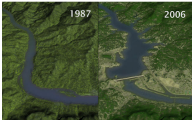
Figure 12: Inundated land effect of building a dam non flowing river current; Indian academy of Environment and Research.
