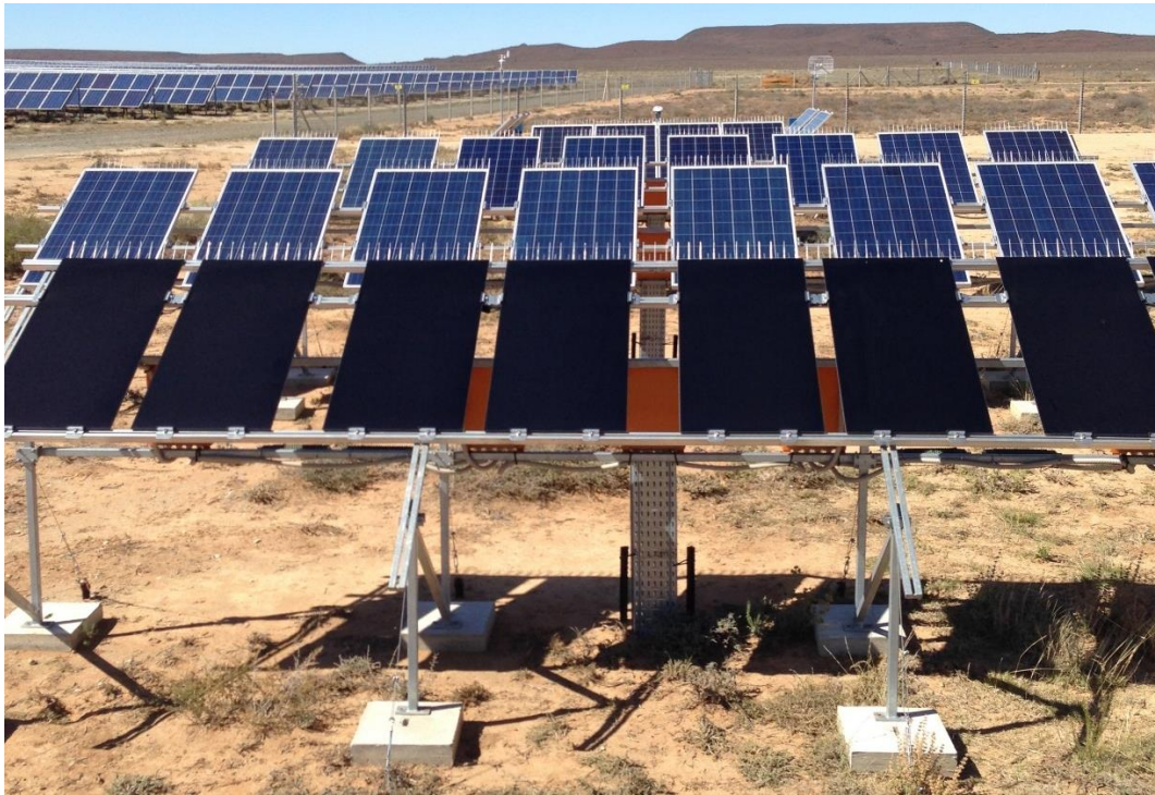
Figure 3-2: Photo of the test facility solar panels, taken from North to South. Thin film modules in front of the silicon modules. In the background to the left is the PV plant. Photo: Mari Øgaard, with permission.
