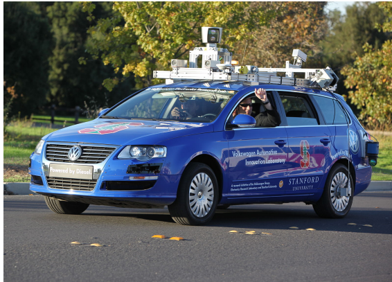
Figure 4.1: "Junior", a self-driving car developed by the Volkswagen Automotive Innovation Lab (VAIL) driving around in a parking lot, 2009 [35].
