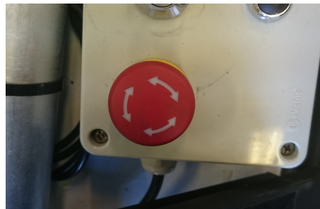
Figure 6.4: Emergency stop button.
