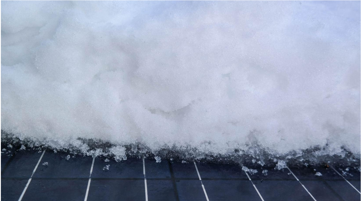
Figure 60. The snow at the bottom of the modules was slushy after the test.
