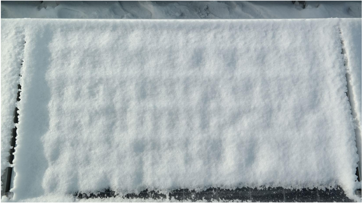
Figure 50. The modules thermal footprint became visible through the snow. The ice cap is seen at the bottom of the photograph.
