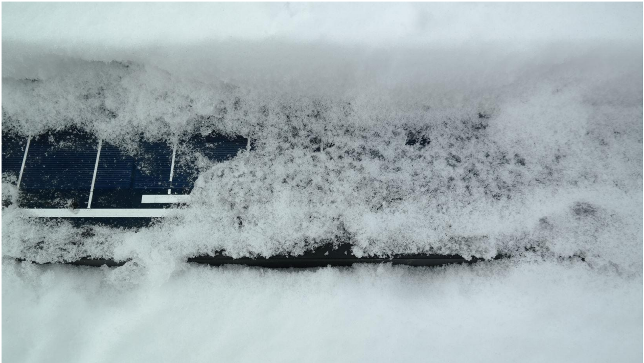
Figure 68. At the end of the experiment it became apparent that an ice sheet had formed at the bottom of the module. The sheet was thin and porous with a surface of something that resembled ice pellets. The ice covered the complete module.
