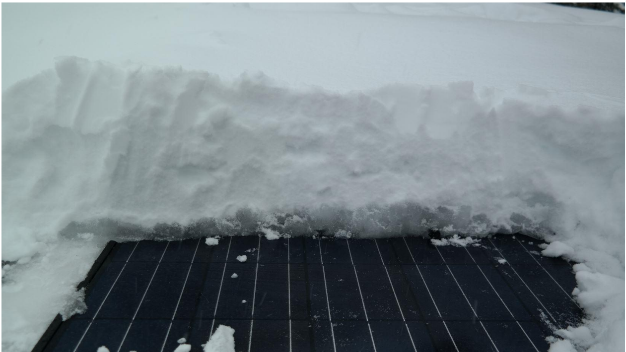
Figure 82. A slush layer formed at the modules surface. The capillary suction of the dry snow created a layer of water-saturated snow.
