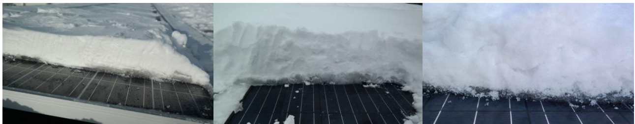
Figure 90. Different cases showing some degree of water saturated snow. Case 2 at ASKO, Case 3 at Nordmarka, and Case 1 at Nordmarka, ranging left to right.
