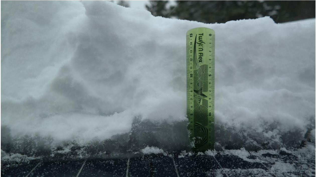
Figure 83. Scale of the saturated layer. The highest point is 5 cm above the module surface.
