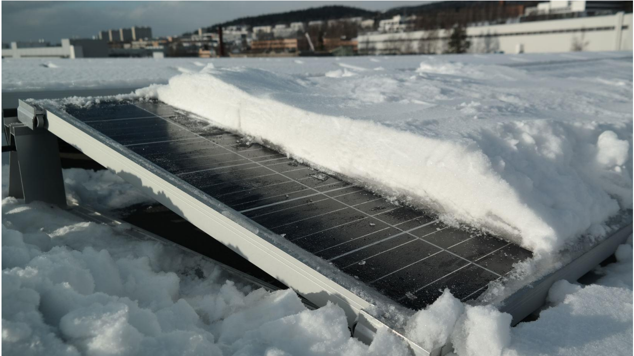
Figure 54. Photograph from a cross section of the snowpack after the experiment. The thickness of the saturated snow-layer is gradually increasing towards the bottom of the module, indicating that water is transported towards the lower edge of the module.
