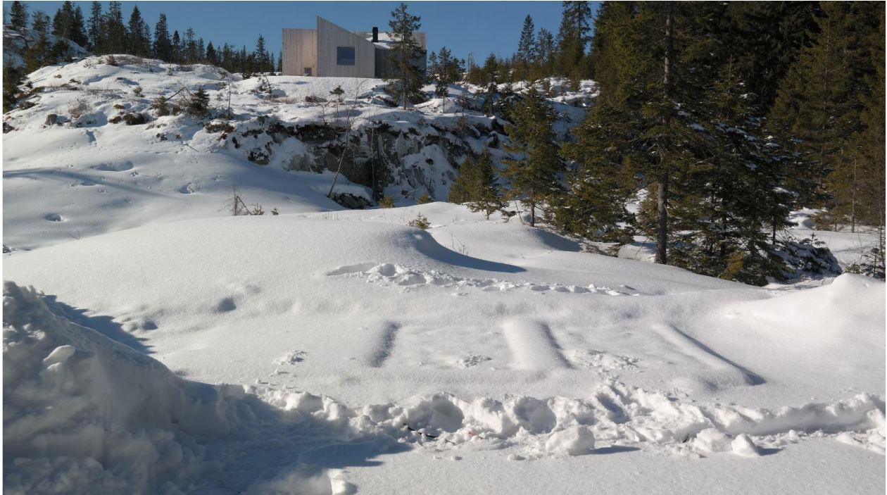
Figure 67. Photograph after the second night of sublimation. A clear dent in the snow can be seen at module 2 and 3. Module 1 is buried beneath the snow next to module 2, appearing as a flat surface.
