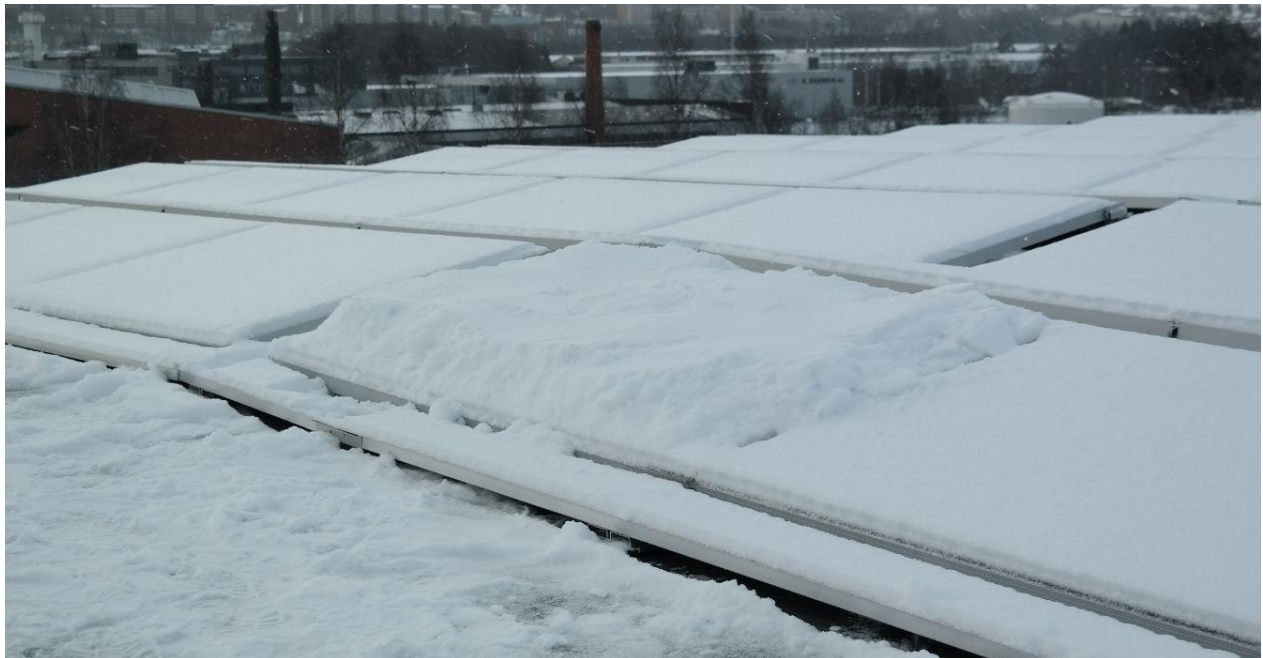
Figure 29. The module with additional snow before testing. The snowpack was not coherent across the modules, leaving the rim exposed.
