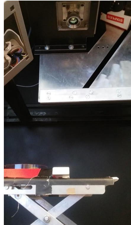
Figure 3-2: The SWIR-camera is shown in the top of the picture, looking down at the sample and spectralon.
