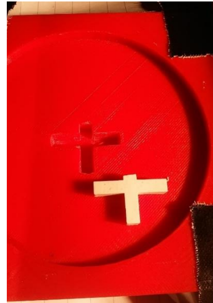
Figure 3-3: 3D-printed plastic mount for the petri dishes.
