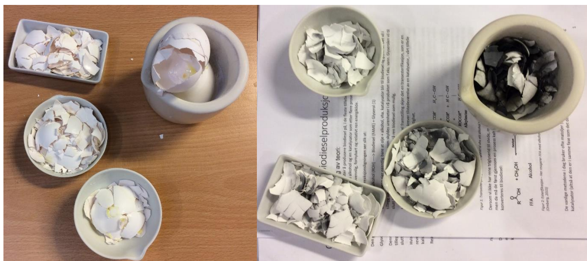
Figure 8: On the left are egg shells from batch 5 that are completely untreated in the mortar and lightly crushed in the crucibles to better fit. On the right are egg shells calcinated at 700\text{ }^\circ\text{C} for 5 h. The black parts of the egg shells are believed to be carbon.
