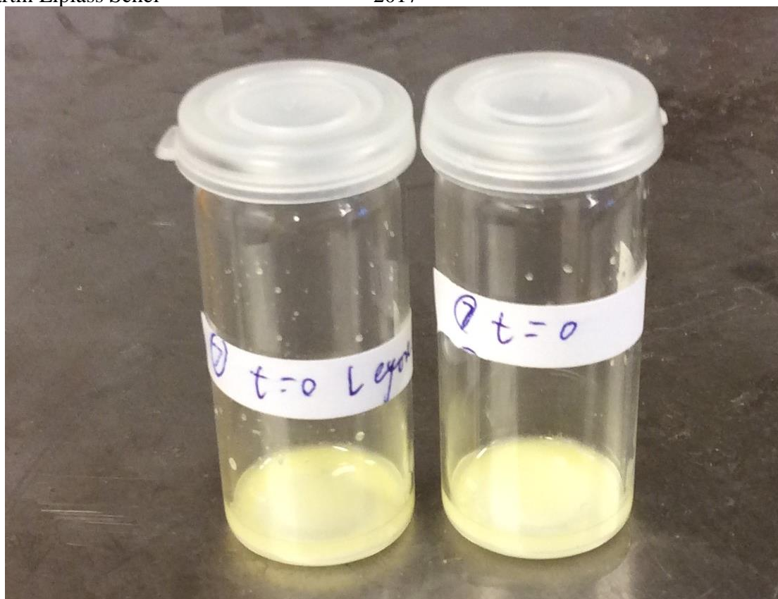
Figure 14: Two labeled sample jars from reaction 7 with lids and content from the reactor taken just before and just after the alcohol was added to the reactor.
