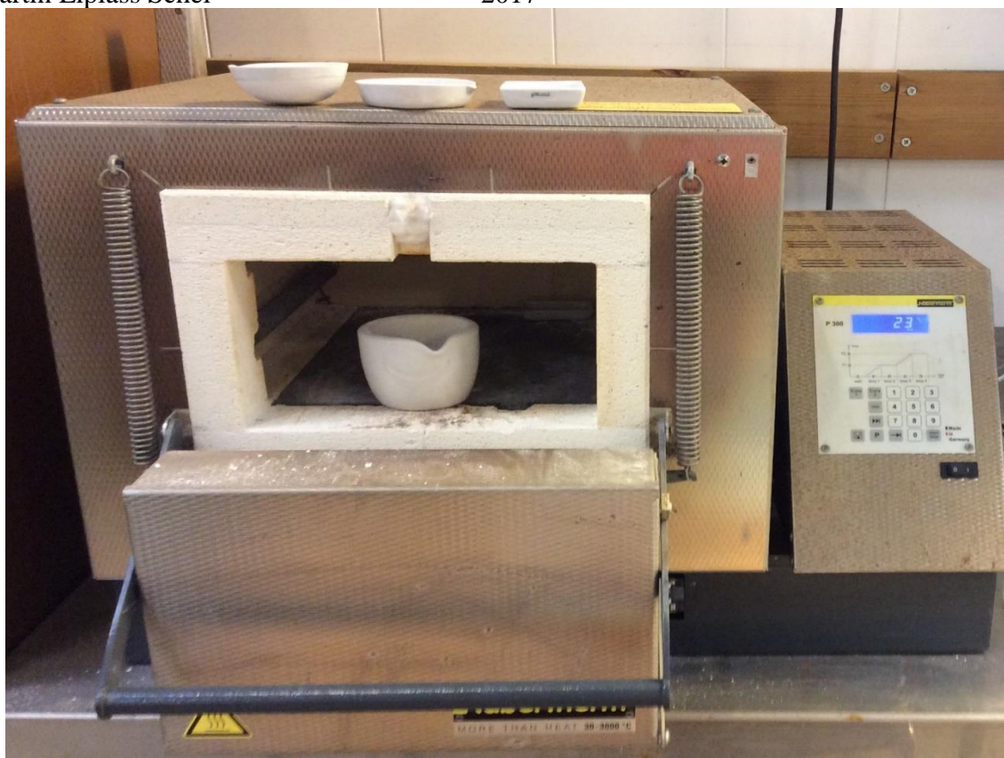
Figure 13: The oven used to calcinate the egg shells and the mortar and crucibles to contain the egg shells during calcination.
