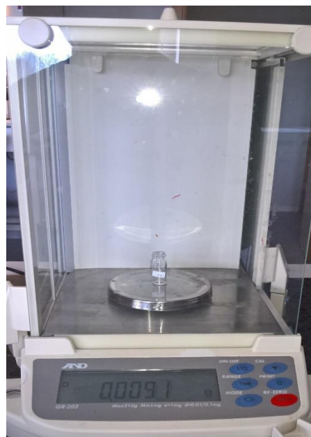
Figure 20: The scale and vial, used to weight the amount of tetradecane and sample that were later analyzed by the GC.
