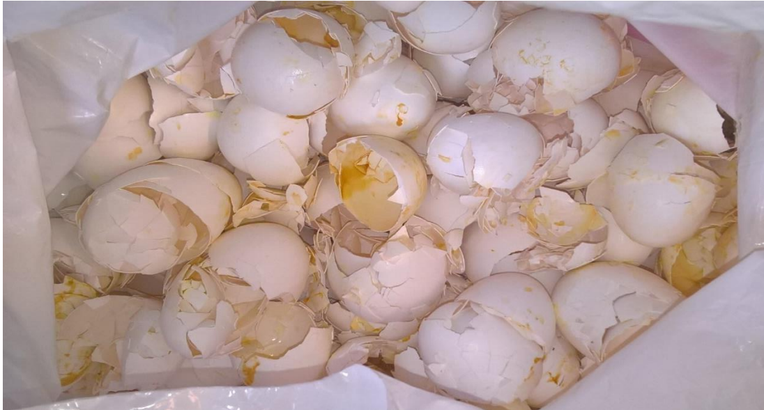
Figure 7: Egg shells as collected from the restaurant kept in a plastic bag and used as batch 4 and 5, rinsed lightly in tap water, and done nothing but lightly crush to fit mortar and crucibles, respectively.
