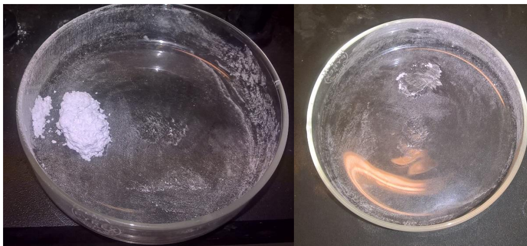
Figure 11: The petri dish used to transport the catalyst, and some catalyst stuck to the bottom caused by glycerol. The petri dish after most of the stuck catalyst was removed and put in the reactor on the right.
