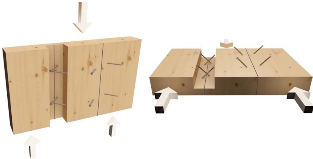
Figure 28: Specimen setup and loading direction.
