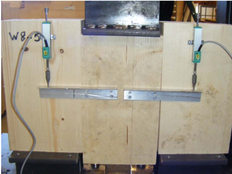
Figure 46: View of the transducers mounted on the specimen.
