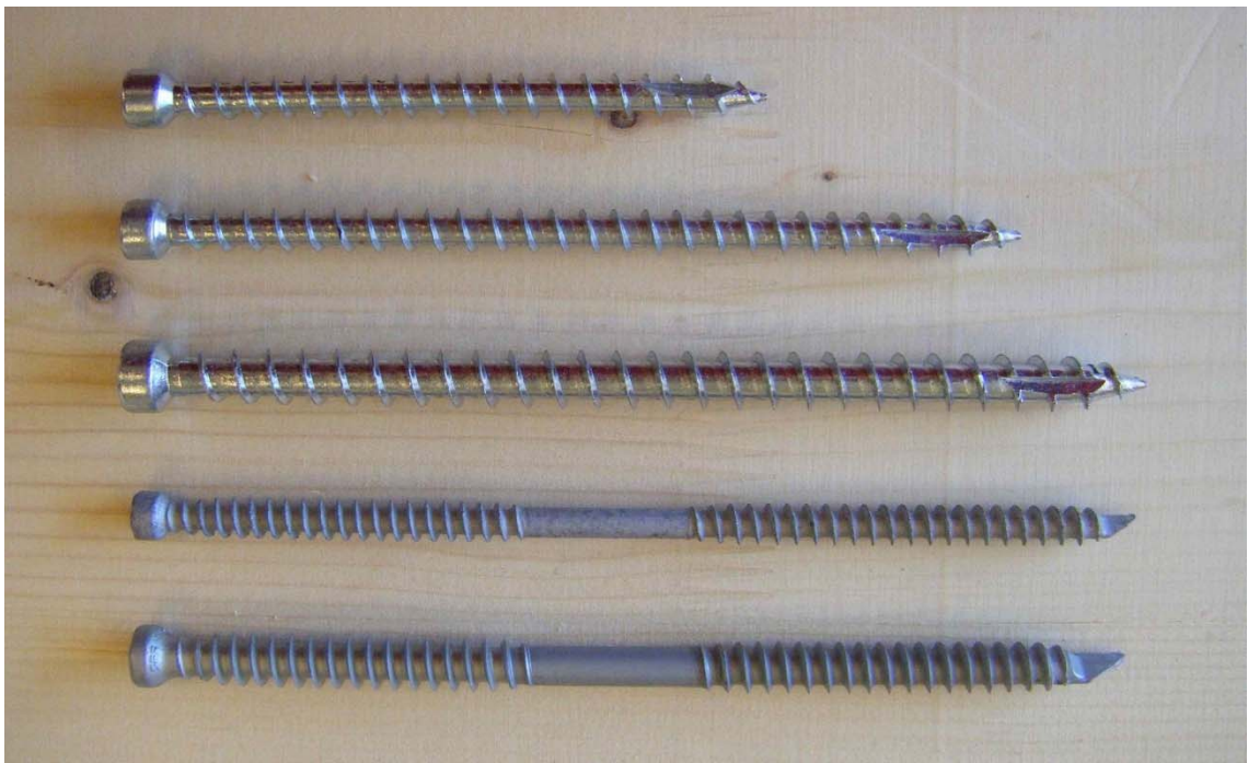
Figure 35: Screws used to join the specimens.
