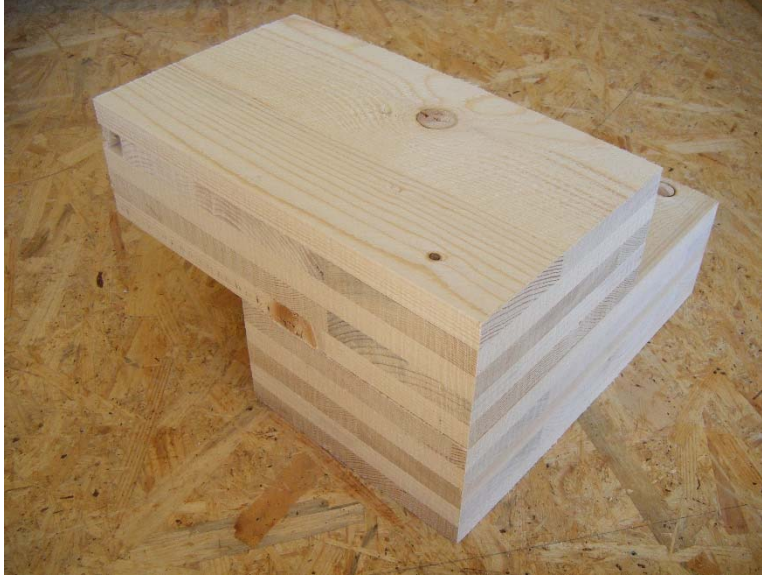
Figure 32: 5 layers, 120mm thick specimen.
