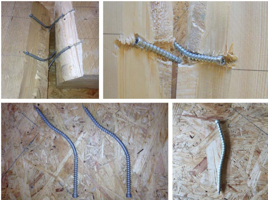
Figure 72: Yielded screws after testing.
