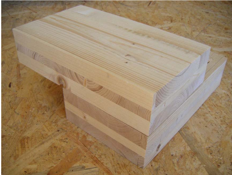
Figure 34: 3 layers, 80mm thick specimen.
