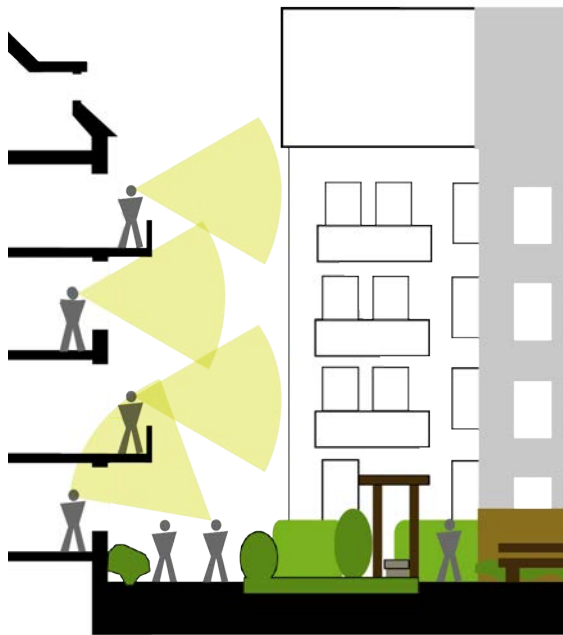
Site section with cone of vision after balcony additions - not to scale
