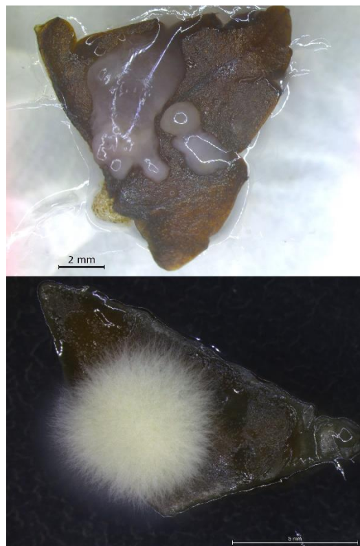
Fig. 5. Examples of A. tumefaciens overgrowth (top) and fungal infection (bottom).
