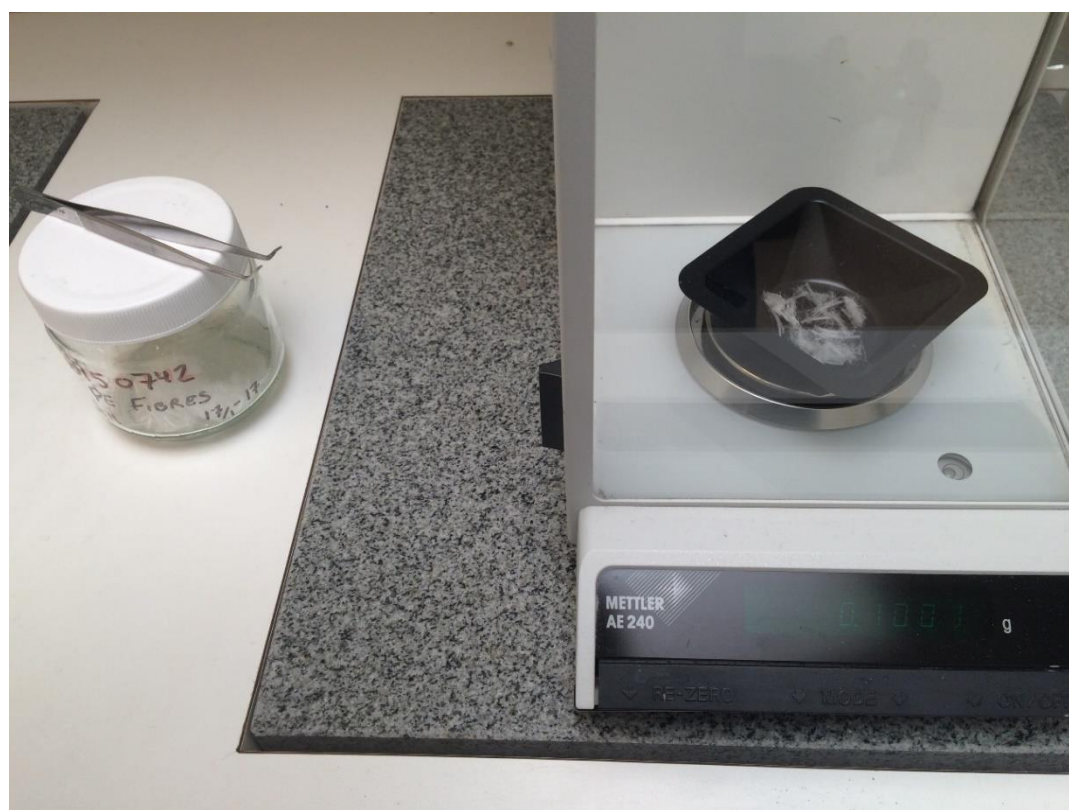
Figure 2: PE fibers shredded into small fragments and 0.1 g weighed on a sensitive scale (0.1 g) for spiking
