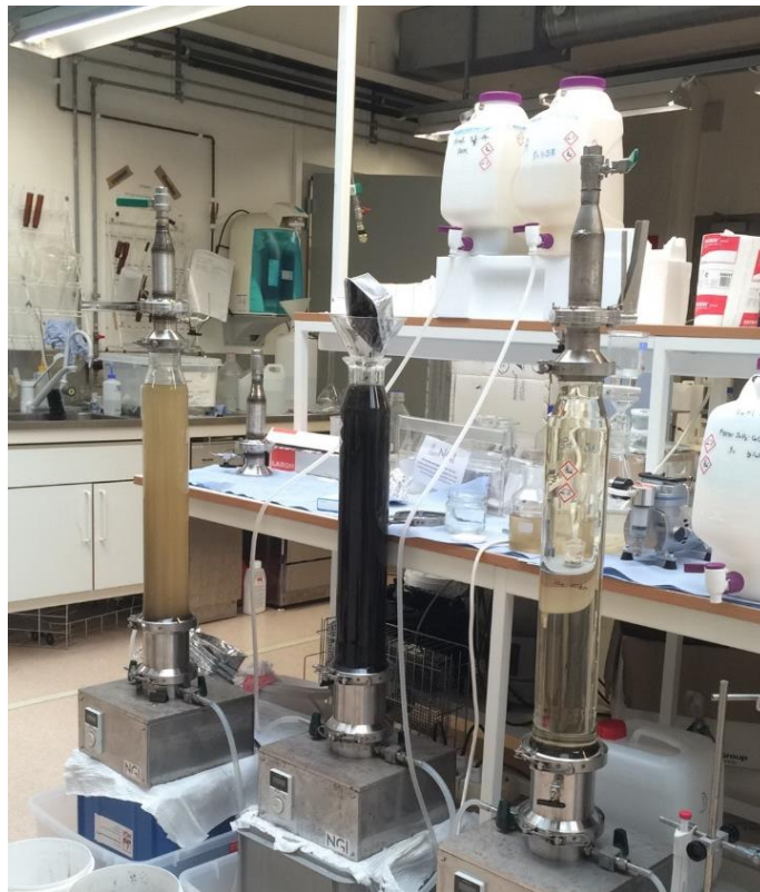
Figure 3: Three Bautas in running condition at NGI. The left-most Bauta (5:1) contains Bygdøy sjøbad beach samples; Bekkelaget sediment introduction in under process in the middle Bauta (50:1); the right Bauta (10:1) is being used for spiking of lab sand
