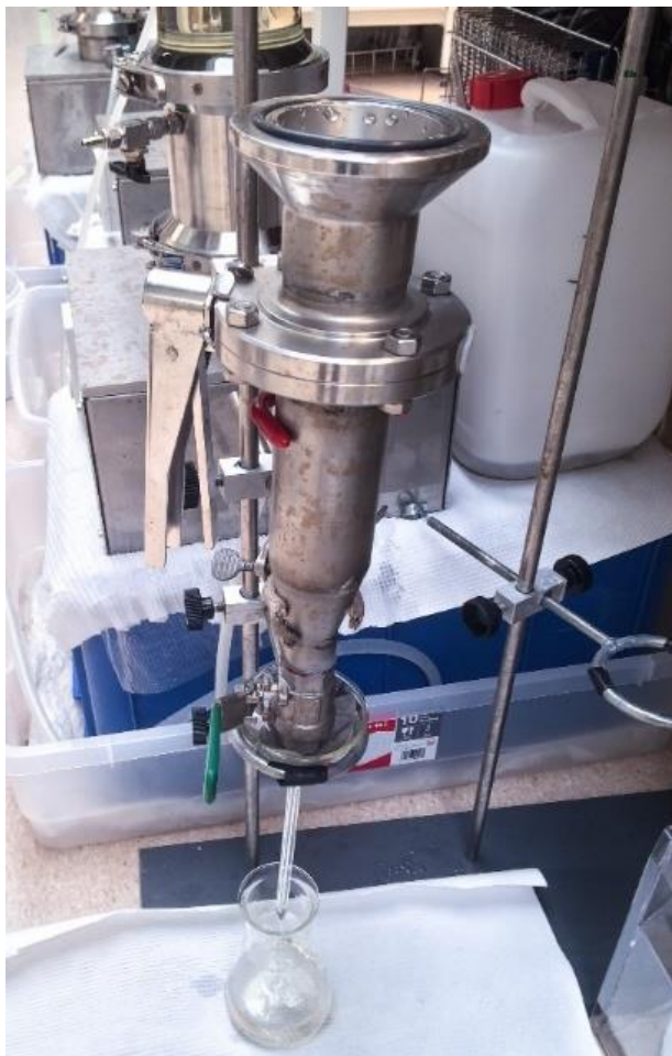
Figure 17: Setup for filtration; sediment chamber is inverted and supported on an iron stand. The glass funnel has a steel mesh (45 \mu\text{m} ) inside. A Schott bottle is kept underneath the funnel, with the stem of the funnel inside the Schott bottle
