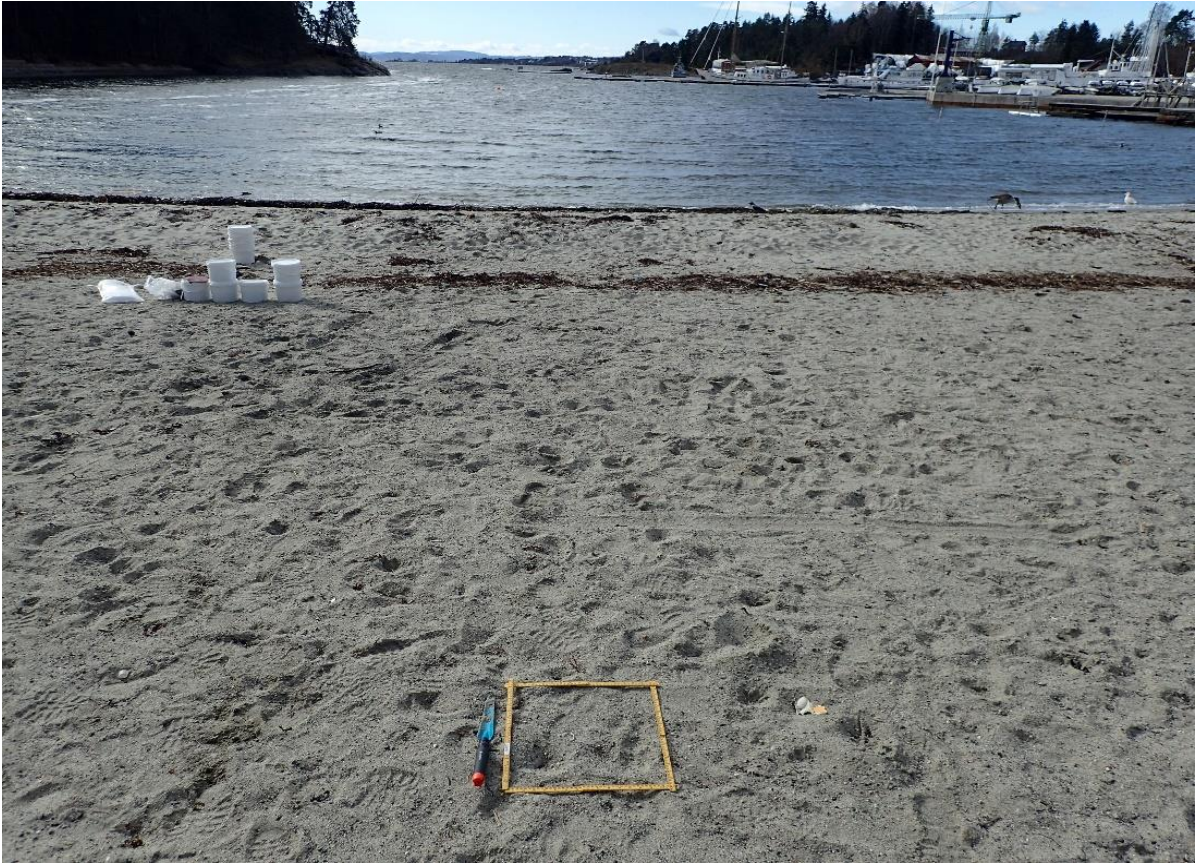
Figure 7: Sampling site in Bygdøy sjøbad. A wooden ruler is placed marking an area of 40*40 cm 2 on one of the sampling points on HWM+6m. Further towards the sea, the HWM can distinguished by the presence of debris accumulated. The HWM-6m, nearest to the sea is noticeable by the accumulation of debris.
