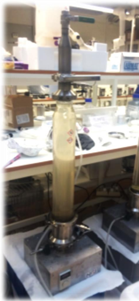
Figure 4: (Left) Bauta Microplastic-sediment separator assembled together and filled with ZnCl_2:CaCl_2 solution
