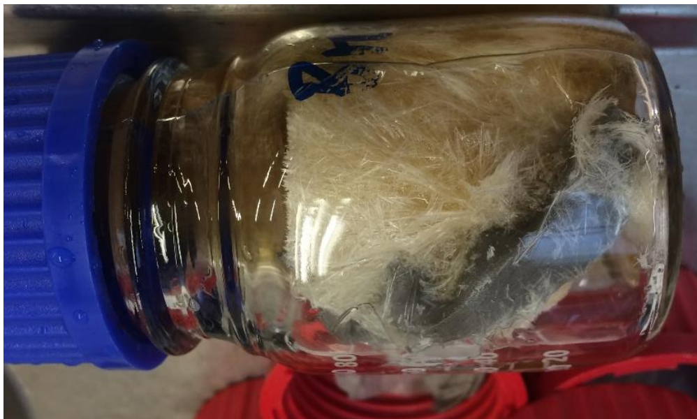
Figure 21: Crystallization of H_2O_2 solution at -20\text{ }^\circ\text{C} when left in freezer for longer than 45 min
