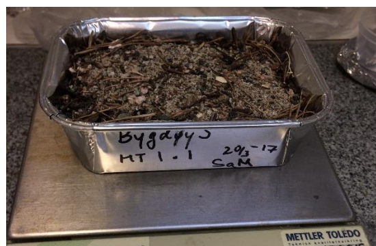
Figure 12: Sample distributed in pre-weighed aluminum trays and weighed before oven-drying at 60 °C, 24h
