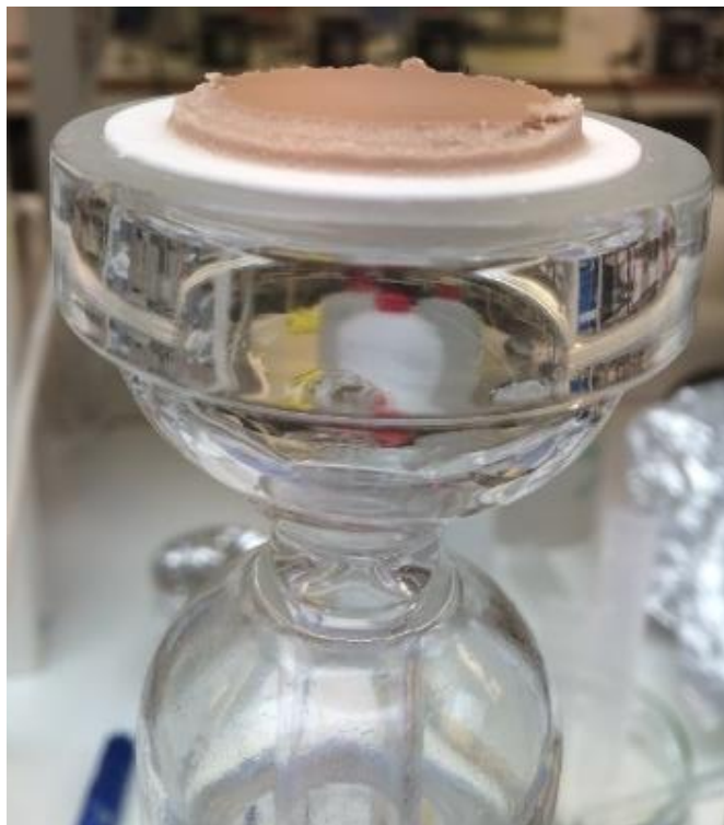
Figure 1: Precipitate filtered out from fresh \text{ZnCl}_2:\text{CaCl}_2 solution on a GF/D filter paper (2.7 \mu\text{m} )
