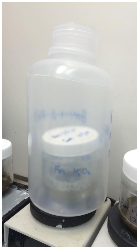
Figure 23: Sample vials kept inside a tall plastic container for safety from spilling of boiling solution and the exothermic mist produced
