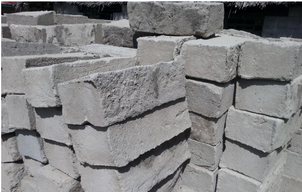
Figure 11. Concrete blocks made of locally available sand and cement at Vanga. Photo: Murungi, E.M. (2017, February 2).
