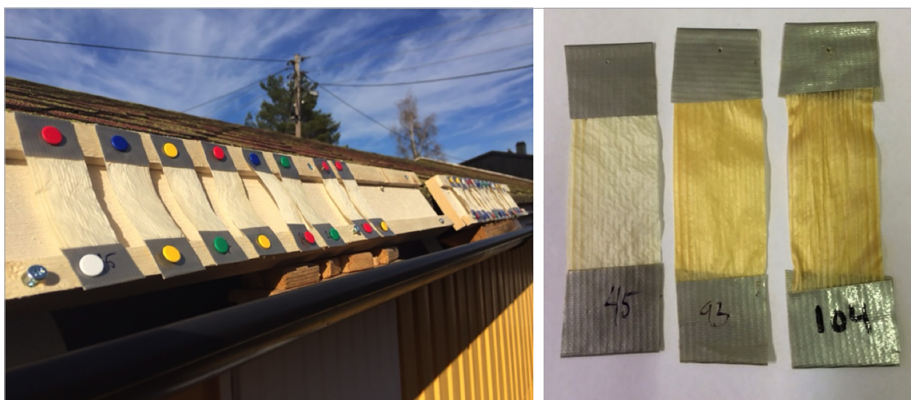
Figure 2. Left: samples exposed outdoors facing south. Right: samples from different sample sets exposed for 1 (no. 45), 10 (no. 93) and 20 (no. 104) days.
