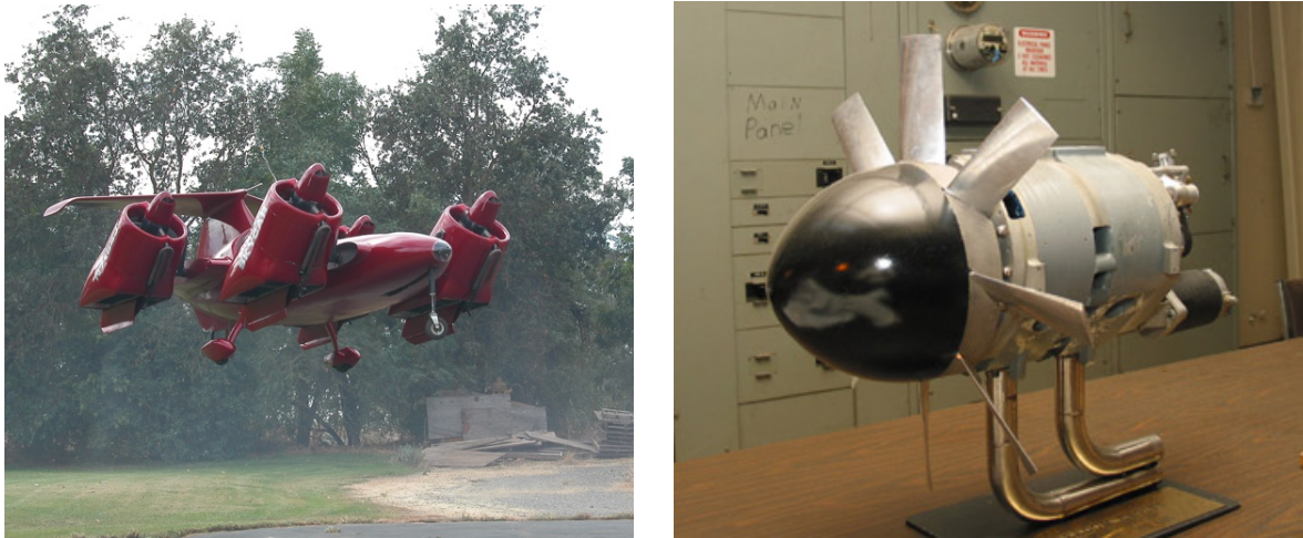
Figure 1.1.4. To the left: Skycar 400 in hovering mode. To the right: Power plant and rotor assembly for Skycar 400. [7]
