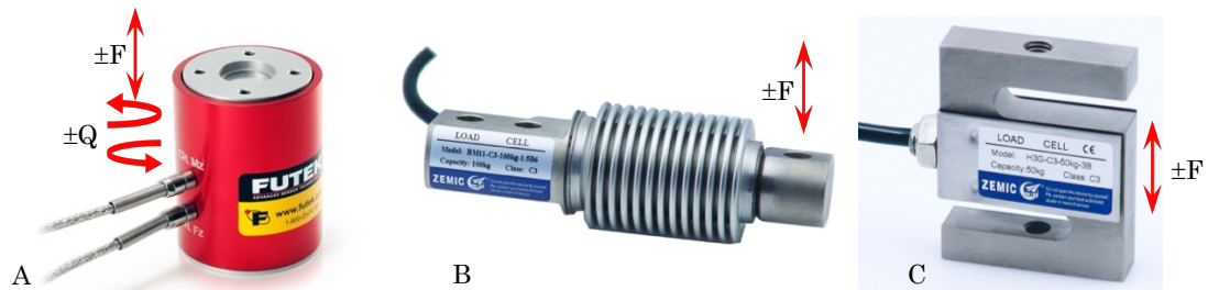
Figure 11.2.1. A: 2-axis load sensor, capable of measuring compression/tension and torque in both directions [37]. B: Bending beam load cell, capable of measuring compression/tension [38]. C: S-type loading cell, capable of measuring compression/tension [38]
