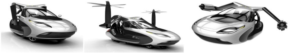
Figure 4.9.4. From the left: 1. TF-X in driving mode with wings and nacelles tucked in to the body. 2. VTOL mode. 3. Flying mode with rotor blades folded in and a ducted fan in the rear generating thrust for forward flight. [27]
