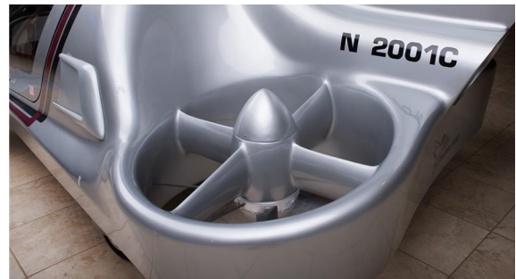
Figure 1.1.3. To the left: Overview of the Sky Commuter. To the right: The fan blades are visible, revealing cord length and angle of attack [6].
