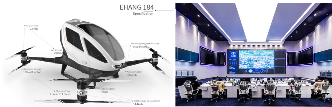
Figure 4.9.1. To the left: Overview of the Ehang 184 with specifications. To the right: Image of the control center in China. [26]
