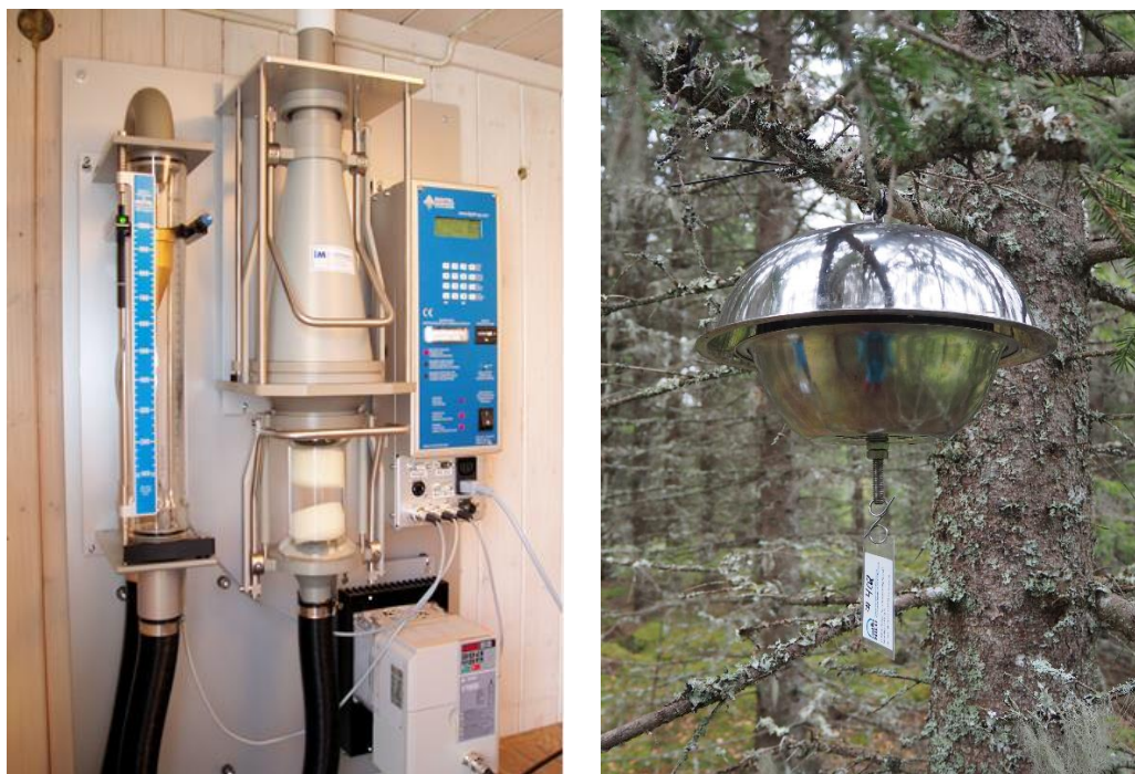
Figure 3: Left: High volume active air sampler (Digitel). Right: PUF based passive air sampler.
