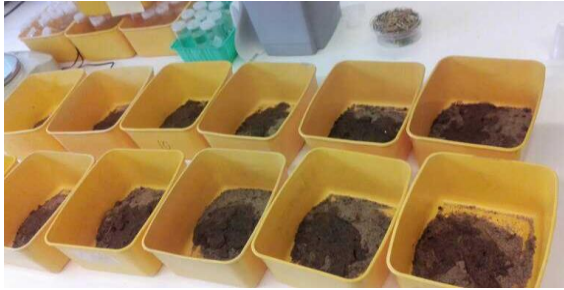
Figure 4 Yellow boxes with sand material before water was added
