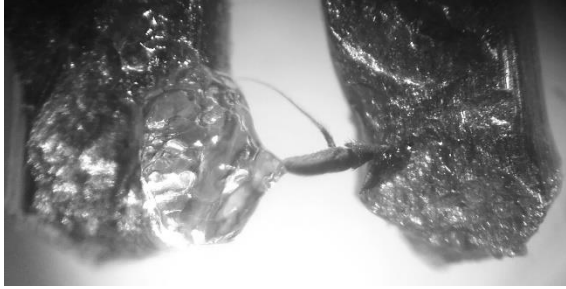
Figure 7 The gel was used to facilitate a good contact between antennae and electrodes. Important to notice is that the antennae were dry, so the pores are not hindered by fluids in detecting volatiles in the puffs of air.
