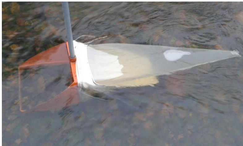
Fig. 5. Photo of the Surber sampler used, illustrating its structure. Note enclosed sides and isolated section of streambed inside frame.
