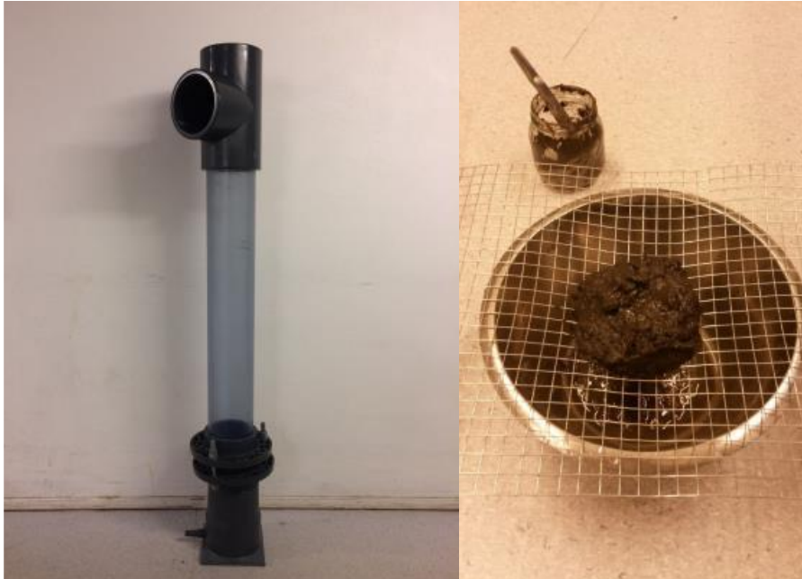
Figure 4a). The elutriation device used for extracting microplastics and b) a sediment sample container with a metal spatula and a 1 cm steel grate on top of a metal bowl. Photo a) personal; and photo b) by Thomas Botolfsen.
