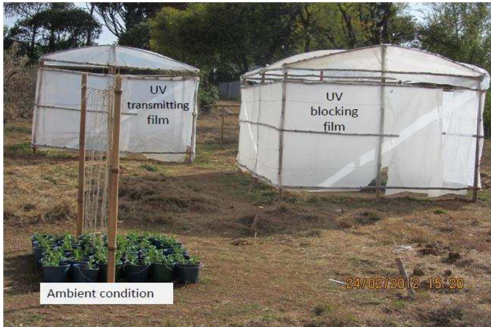
Fig. 6. Experimental layout established to evaluate the impact of UV-transmitting and UV-blocking films on the growth and productivity of commercial pea ( Pisum sativum cv. Cascadia) at higher (2800 masl) and lower (1700 masl) altitude of southern parts of Ethiopia during the dry (January – April) and wet (April – June) season in 2012.
