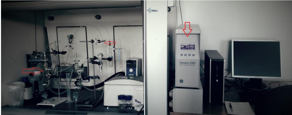
Figure 9. The nitric oxide (NO)-Analyzer (NOA) (Sievers NOA 280i) and its chemical set up. Left panel: Gas - over, and - under pressure through plastic & glass tubes make out the system for determining the nitrite concentrations (nM to mM concentrations). To the right: the NOA (the tallest, white box with blue display). A sample is injected manually into a rubber-sealed glass-system. There, nitrite traces in sample will react with a reducing agent (NaI in 50 % acetic acid) which converts nitrite into NO. Inert N_2 bubbles through the reducing agent, and thus carries the NO through the glass- and plastic wires. At the endpoint, the NOA detects NO through chemiluminescence.
