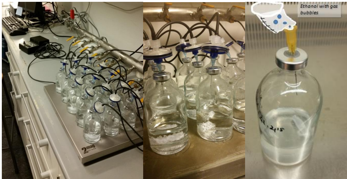
Figure 6. Helium-wash and pressure adjustment. Left: Experimental flasks being Helium washed after autoclaving. Middle: Bubbles forming during evacuation are shown on magnet bars at bottom of the serum flasks. Right: Headspace in a serum flask being adjusted to pressure equal to lab-environment.
