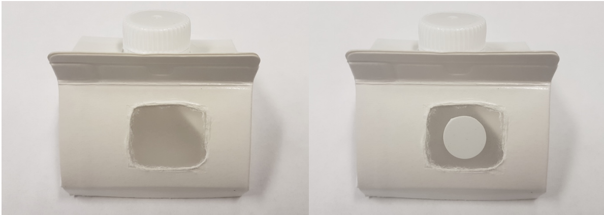
Figure 6: Exposure of EVOH gas barrier after removal of outer PE and board layer on gable top carton for allowing septum placement directly on gas barrier.
