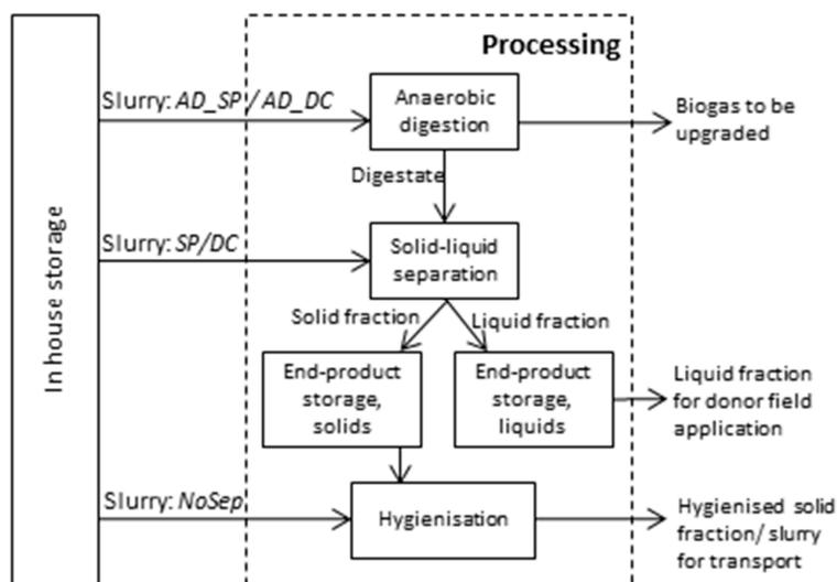
**Figure 3.** An overview of the processes included in the main process of “Processing” in Figure 2, indicated by the dotted line. The figure shows the processes (boxes) used under the different scenarios (in italics) to process slurry from in house storage and how the processes are connected by flows (arrows).
