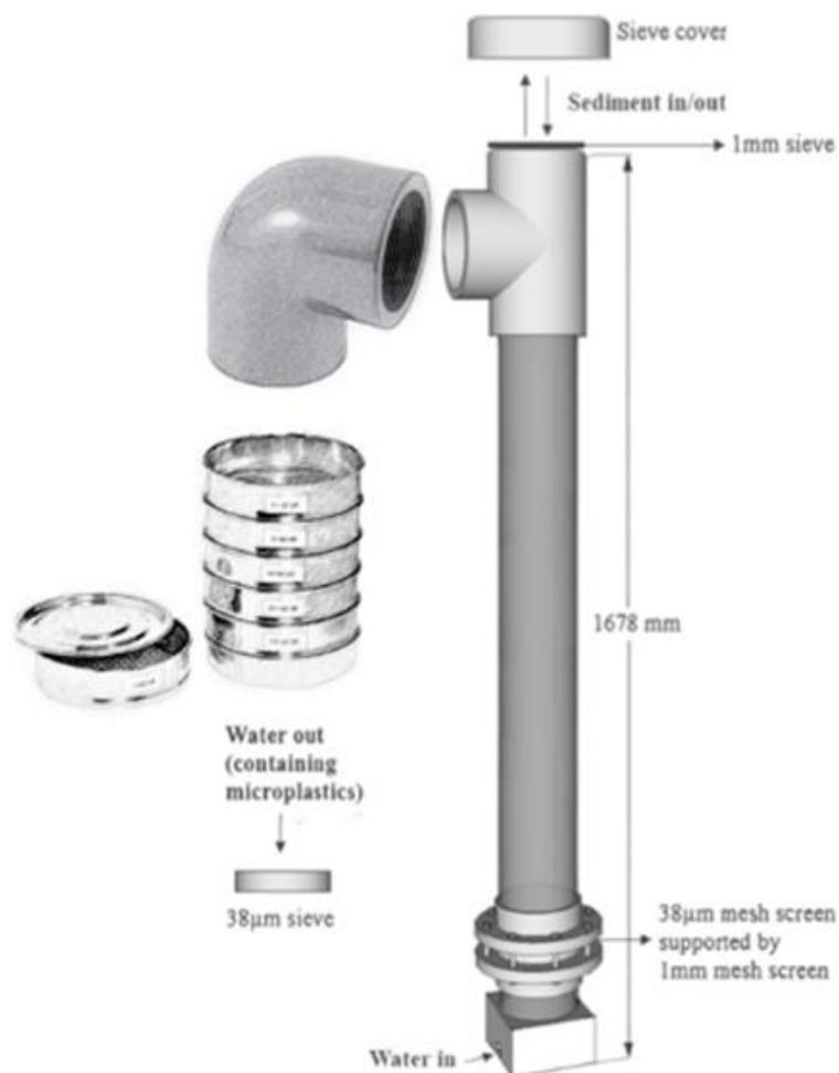
**Fig. 10.** Elutriation device with new suggested components to decrease possible air contamination of samples and to increase microplastic retention. A 90° elbow joint attached to a system of several sieves in a descending order of mesh size (Modified from Claessens et al. 2013).
