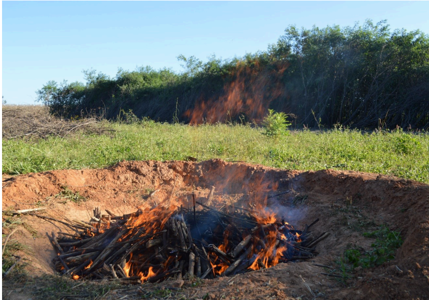
Figure 3: Test of Flame curtain kiln. Picture taken by Vegard Martinsen in Mkushi, Spring 2015.
