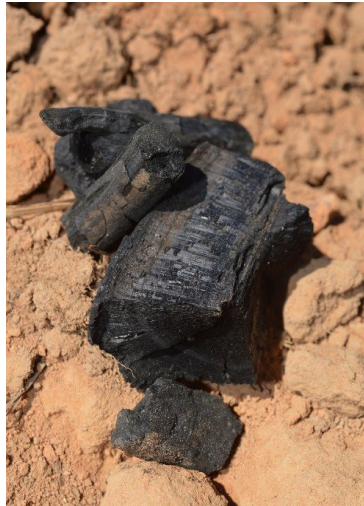
Figure 2: PP BC made in flame curtain kiln in Mkushi, Spring 2015. Picture taken by Vegard Martinsen.
