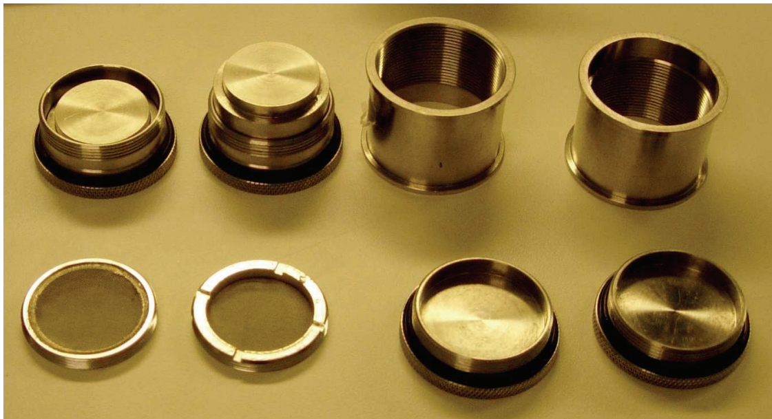
Figure 5. Sample cups with filters and lids for top and bottom.
